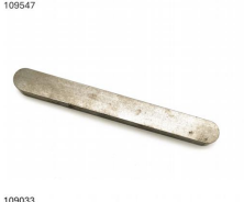
109547 feather key DIN6885 A18x11x160 Passfeder 18h9x 11h11x160 DIN6885A C45K
