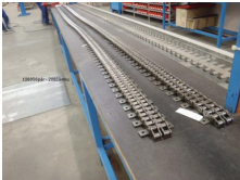
108956 roller chain double 16B-2 DIN8187 208 li Rollenkette 2-fach 16B-2 DIN8187 208GI.
