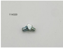
114320 lubricat.nipple M6x1 45° DIN71412B Schmiernippel M6x1 45° DIN71412B
