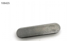
108425 feather key DIN 6885 A 12x8x50 Passfeder 12h9x 8h11x 50 DIN6885A C45K
