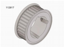
112817 HTD toothed belt disc TL 34-5M-15 3F HTD Zahnriemenscheibe TL 34-5M-15 3F
