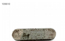
109610 feather key DIN 6885 A12x 8x 45 Passfeder 12h9x 8h11x 45 DIN6885A C45K
