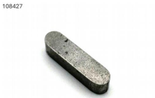
108427 feather key DIN 6885 A 5x5x 20 Passfeder 5h9x 5h9x 20 DIN6885A C45K
