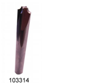
103314 hard metal milling cutter ø 3,7R2,0 Fräser-R ø 3,7R2,0 SL 2 GL 64 DS 8h6 Z4
