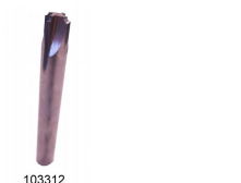
103312 hard metal milling cutter ø 5,7R1,0 Fräser-R ø 5,7R1,0 SL 1 GL 64 DS 8h6 Z4
