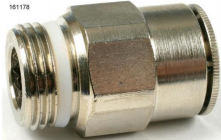
161178 straight pipe fitting 12-3/8 with seal Steckverschr. G 3/8"-ø12 SW19 MS vern.
