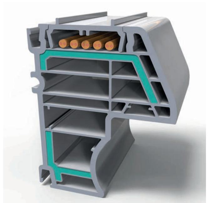
**Fig. 4.** Door profile of a chest freezer: hereby, Ultradur replaces a metal stiffener, which eliminates the need for an electrical heater in the profile to prevent condensate formation on the outer surface. This improves the freezer's energy efficiency.
