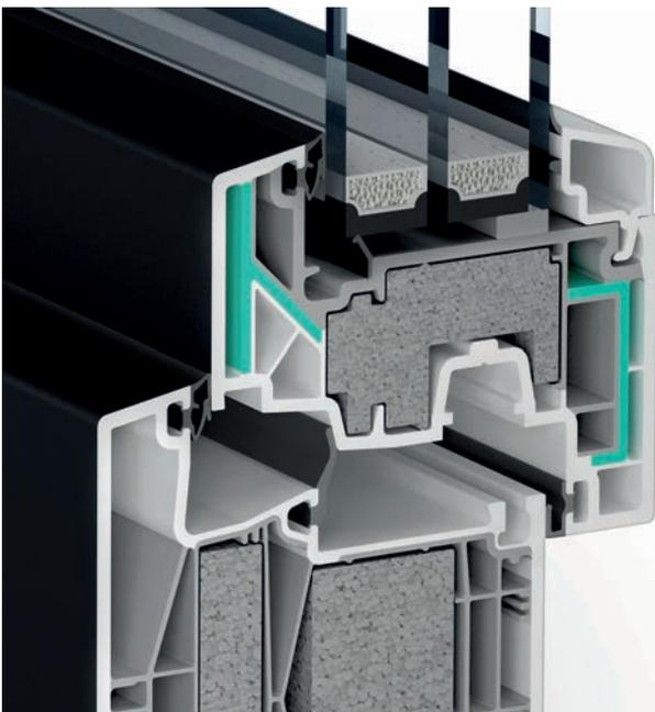
**Fig. 3.** Ultradur B4040 G11 HMG HP can be used instead of steel to stiffen rigid PVC profiles. The result is a lower permanent deflection after one-sided heating. Moreover, thermal conductance is reduced. This permits large, energy-saving windows, also with dark-colored profiles.
